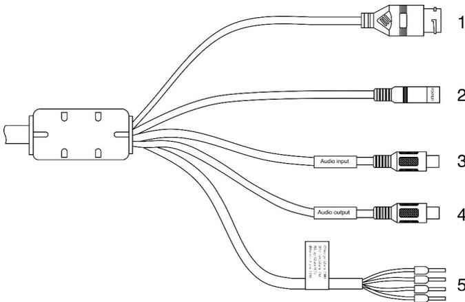
Figure 1-2 Simple multi-head cable (optional)
